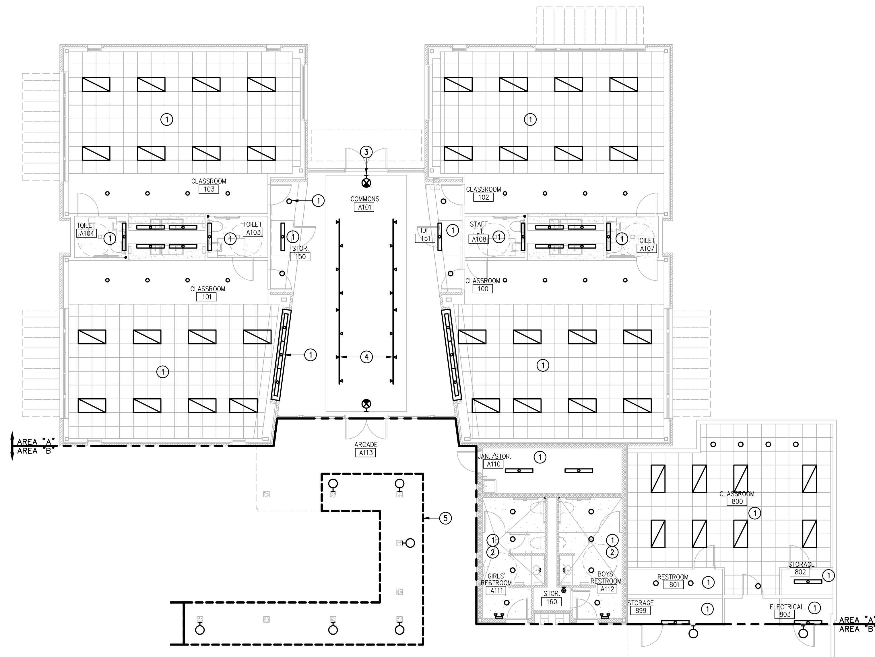
IDEA CARVER DEMOLITION - LIGHTING PLAN (BUILDING A) 01 SCALE: 1/8" = 1'-0"
